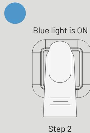
2.3 Place the finger that needs to be registered on the sensor. Continuously press the fingertip 10 times on the fingerprint sensor until the “blue light” turns on. Note that Bluetooth-enabled locks may require only 5 additional presses.
